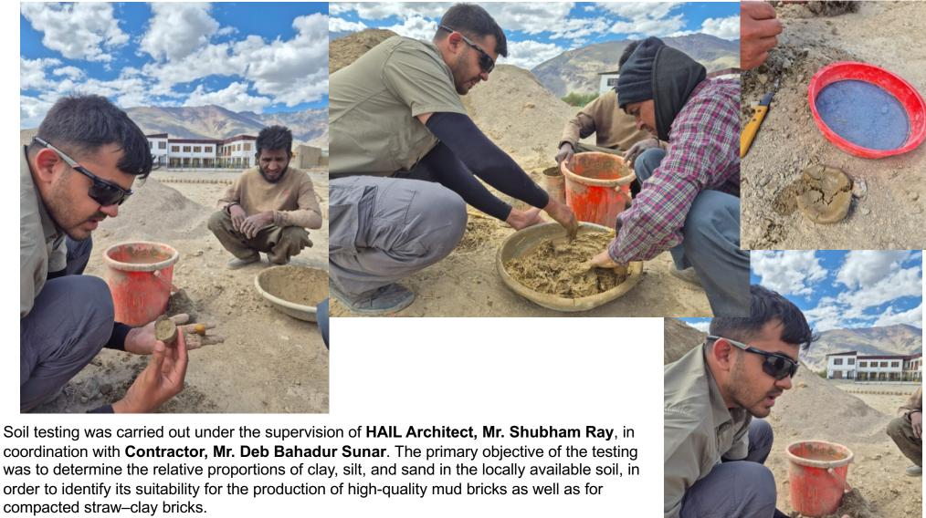
coordination with Contractor, Mr. Deb Bahadur Sunar. The primary objective of the testing was to determine the relative proportions of clay, silt, and sand in the locally available soil, in order to identify its suitability for the production of high-quality mud bricks as well as for compacted straw-clay bricks.
